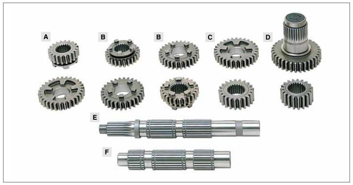
All 5 speed Sportster gears are made from high nickel alloy steel. Gears are then heat treated and shot-peened to give maximum durability and strength. Also, where applicable, drive
