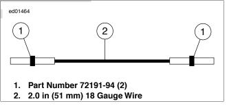
Figure 2-6. Diagnostic Test Wire
