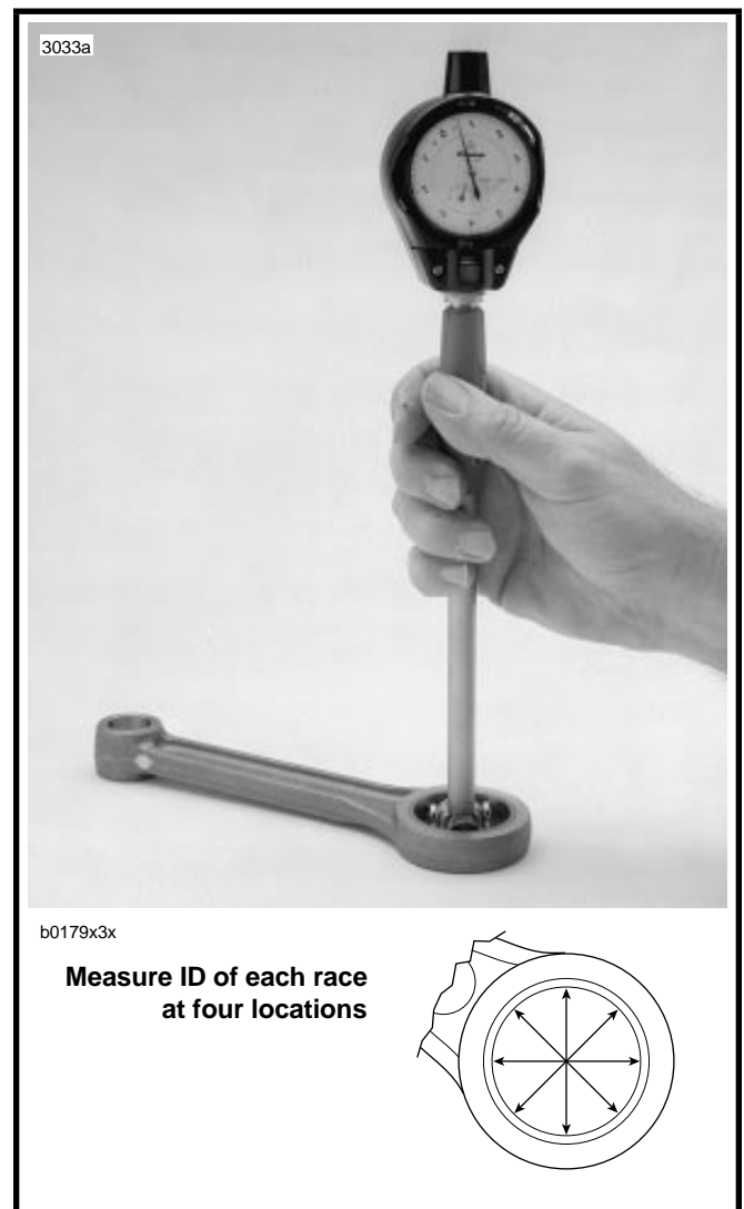
Figure 3-73. Measuring Connecting Rod Race Inside Diameter
