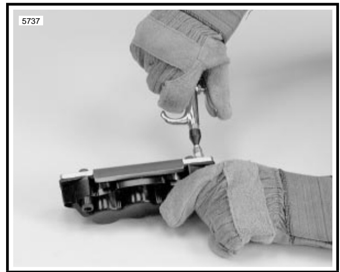
Figure 2-21. Removing Brake Caliper Pistons Using Brake Caliper Piston Remover (Part No. B-42079)
