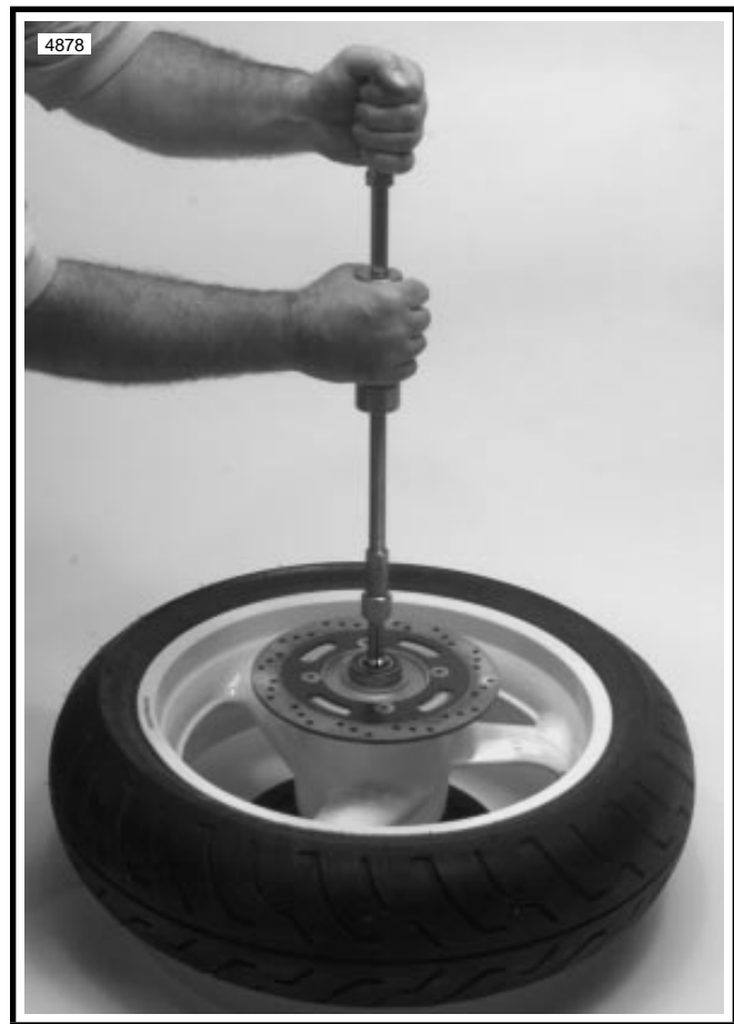
Figure 2-10. Removing Wheel Bearing Using Bushing/ Bearing Puller (Part No. HD-95760-69A) and 1 1/8 in. Collet (Part No. HD-95769-69)
